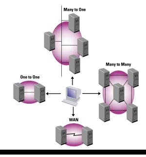
RepliStor can be configured to replicate data in any environment as shown in the illustration to the left. It also is ideal as a business continuance/disaster recovery solution when data is transmitted over a Wide Area Network to a replicated site.
